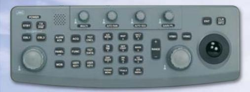
The combination of push button and analog controls of the keyboard ensure a logical, precise operation. The newly developed processor technology ensures that selections are instantly displayed on the screen.
